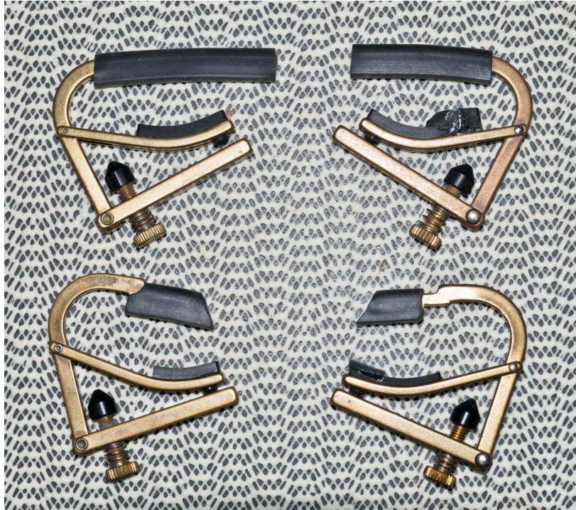
Figure 1. Shubb Full and Partial Capos. Upper left: full or 6-string capo (Shubb C1). Upper right: modified “4-string outer” banjo capo (Shubb C5b-r). Lower left: Esus4 “E-gad” 3-string capo (Shubb C7b). Lower right: a “cut” (modified) Esus4 “E-gad” capo (Shubb C7b) that capos only two middle strings. The hinge side “hump” of the Esus4 allows the capo to clear the outer string so on the “middle-2” capo I’ve cut away some of the neck-side rubber pad and filed the brass down to clear two outer strings. Note the added rubber on the neck side of the banjo capo, and to the neck side of the “middle-2” capo to better fit the curve of the neck.
