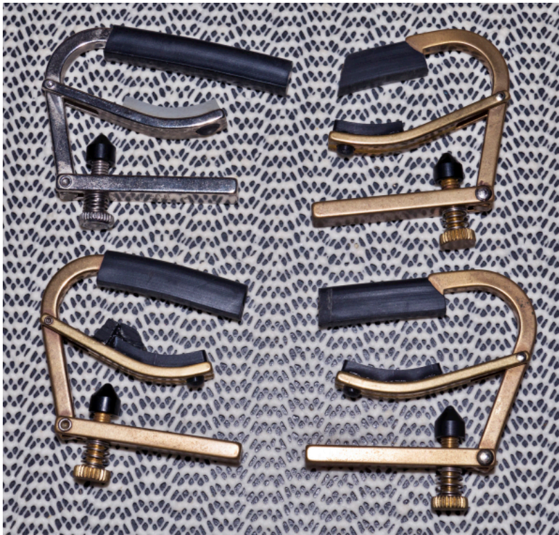
Figure 1. Shubb Full and Partial Capos. Upper left: a full or 6-string capo (Shubb C1). Upper right: an Esus4 “E-gad” capo (Shubb C7b). Lower left: a modified banjo capo (Shubb C5b-r). Lower right: a modified, “cut” 5-string capo (Shubb C8b). The hinge side “hump” of both the Esus4 and the modified 5-string (drop E, with end cut to clamp only four inner strings) allow the capo to clear the outer string. Note the added rubber on the neck side of the banjo capo (a radius version shown here) to fit the neck better—without the added rubber, these capos tend to tip or pull forward on the hinge side and will not clamp the outer string properly.
